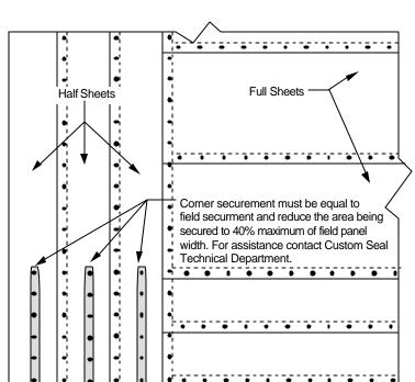
As an option, comer enhancement may be accomplished by installing additional rows of securment through the half sheets and then striping in those rows of securement with PVC flashing installed to Custom Seal specification.
