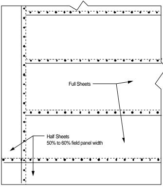
All Custom Seal PVC Mechanically Attached Systems require half sheet perimeter securement. A half sheet width of up to 60% of the width of the field panels may be used. Half sheet securement is equal to the membrane securement used in the field of the roof. See the Mechanically Attached PVCCode Matrix for fastener and spacing requirements. If the project must meet Factory Mutual criteria refer to detail 42.04-3 and contact Factory Mutual for review.
