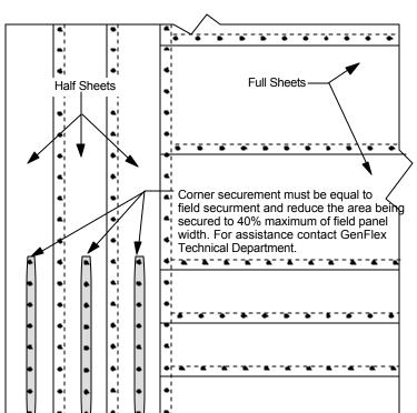
As an option, corner enhancement may be accomplished by installing additional rows of securment through the half sheets and then striping in those rows of securement with either TPO flashing or TPO Cover Tape installed to Custom Seal specification.
