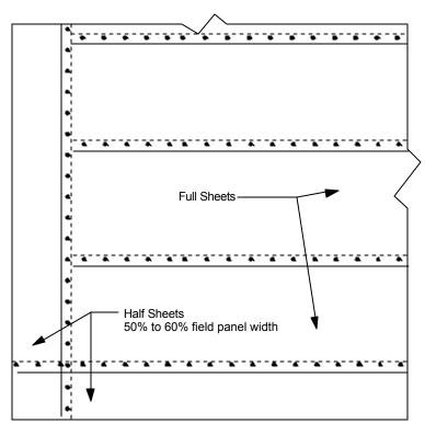
All Custom Seal TPO Mechanically Attached Systems require half sheet perimeter securement. A half sheet width of up to 60% of the width of the field panels may be used. Half sheet securement is equal to the membrane securement used in the field of the roof. See the Mechanically Attached TPO Code Matrix for fastener and spacing requirements. If the project must meet Factory Mutual criteria refer to detail 42.04-3 and contact Factory Mutual for review.
